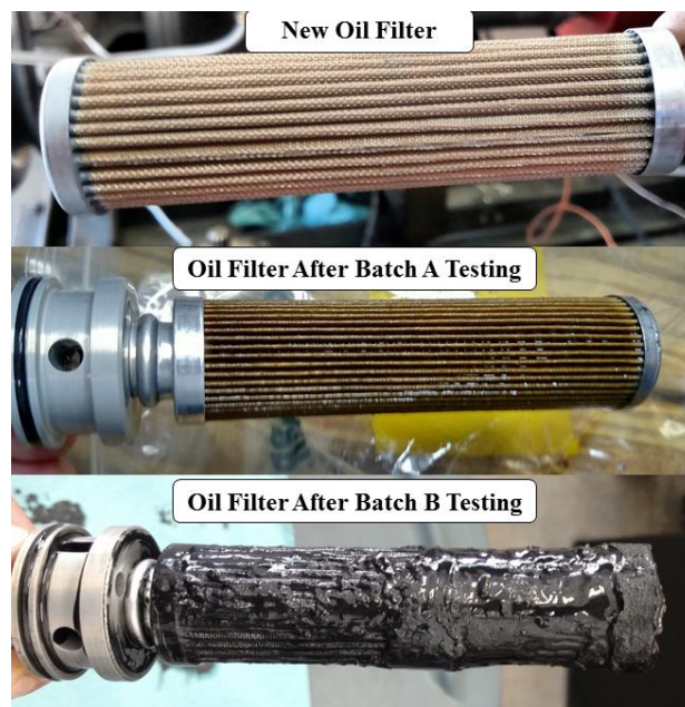
FIGURE 3.10 OIL FILTER BEFORE AND AFTER TESTING
